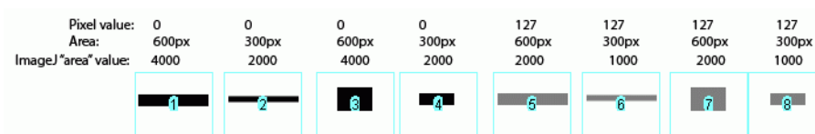
Figure 26. Image-J will return similar area values when bands have equivalent numbers of pixels of equal darkness, but vary in shape.
